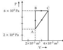
In process AB, 400 J of heat is added to the system and in process BC, 100 J of heat is added to the system. The heat absorbed by the system in the process AC will be
