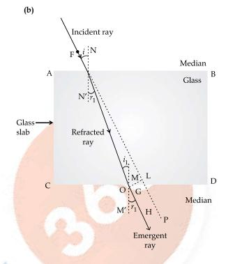
EF is the incident ray and GH is the emergent ray, which is parallel to the incident ray.
